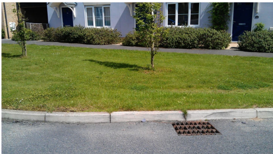
Image: Example of missed opportunity. Flows enter gully pot rather than being directed into greenspace. The gully pot could be sealed and rainfall runoff from the road could be directed into the adjacent green space.
